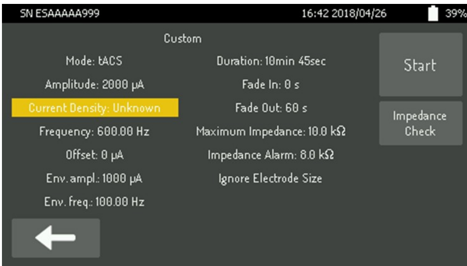
Figure 59. Current density is unknown as electrode size has not been entered. Stimulation can still start.
