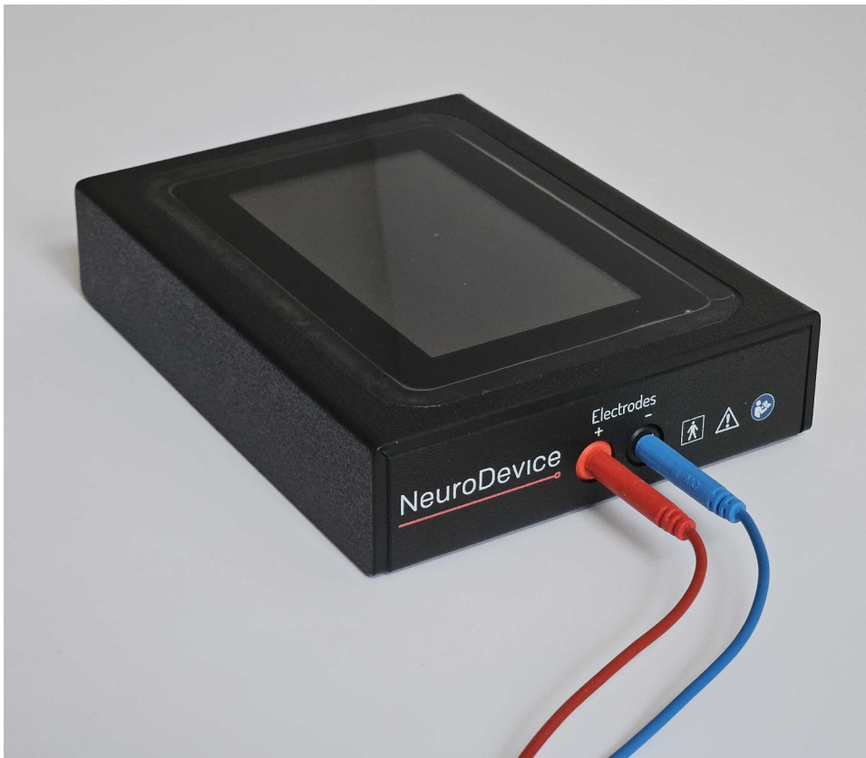
Figure 7. Correct electrodes cables connection
