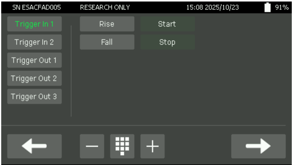
Figure 98. Input triggers settings screen.
