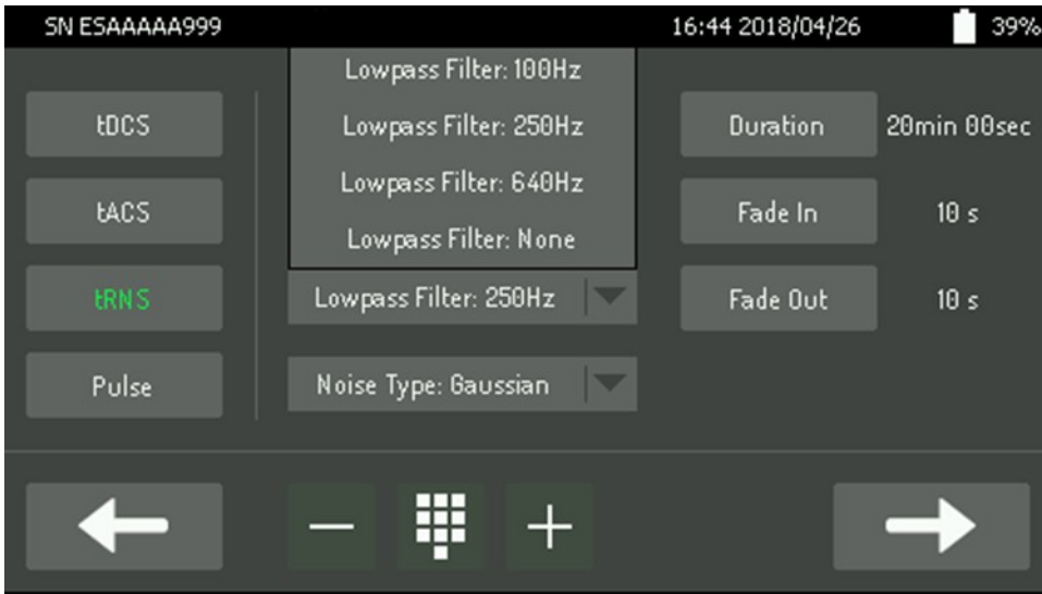
Figure 35. Setting lowpass filter for tRNS.
