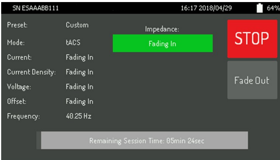
Figure 65. Stimulation screen showing mode, impedance bar. Measured values are shown as "Fading in" or "Fading out" during the fade in and fade out periods.
