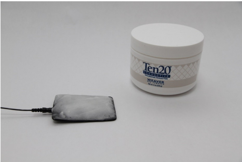
Figure 9. Arrangement of the gel on the electrodes.
