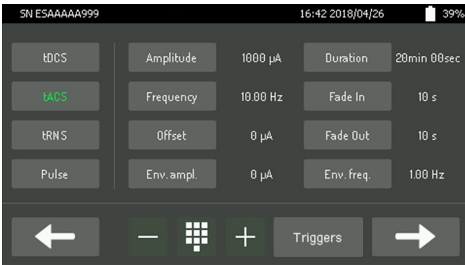
Figure 13. tACS highlighted showing different parameters.
