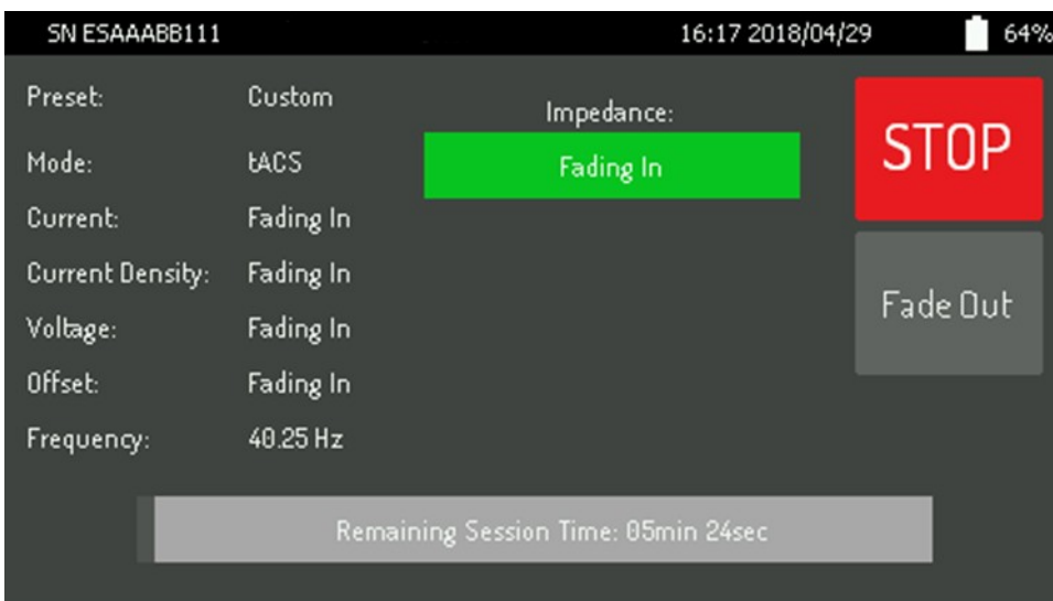
Figure 62. Stimulation screen showing mode, impedance bar. Measured values are shown as "Fading in" or "Fading out" during the fade in and fade out periods.
