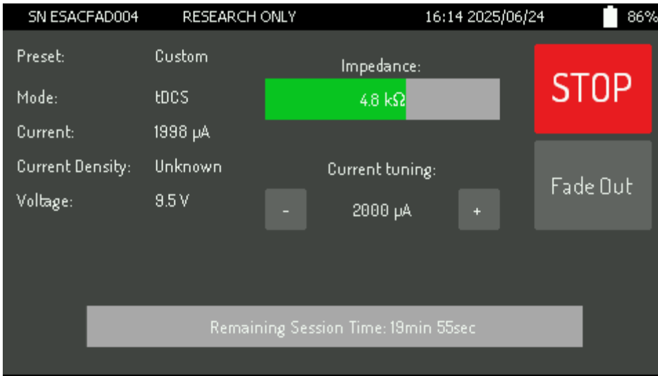
Figure 50. Stimulation running in test mode. The + and - button allows to change current intensity in real time.
