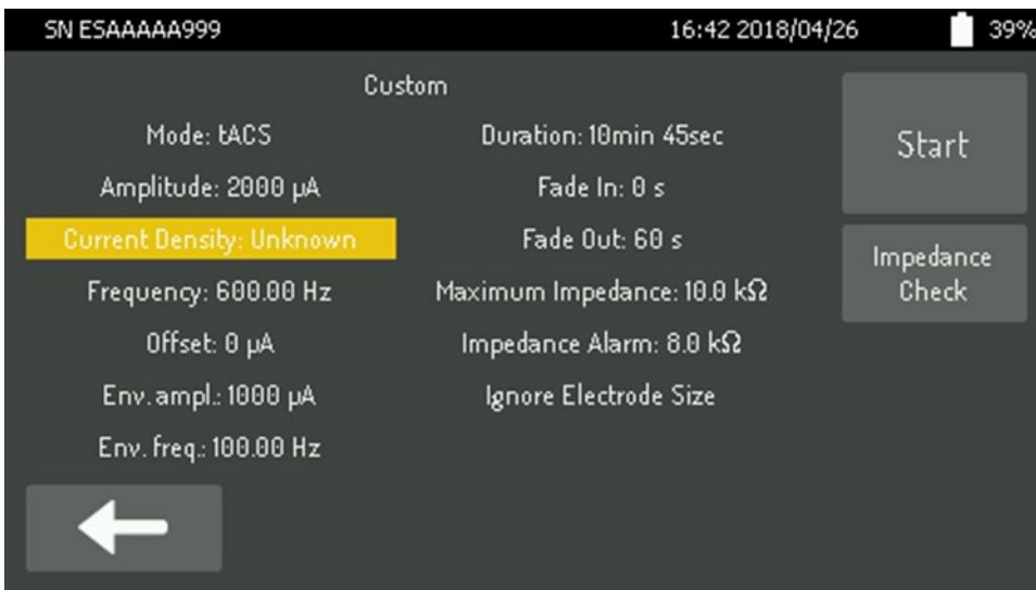
Figure 56. Current density is unknown as electrode size has not been entered. Stimulation can still start.
