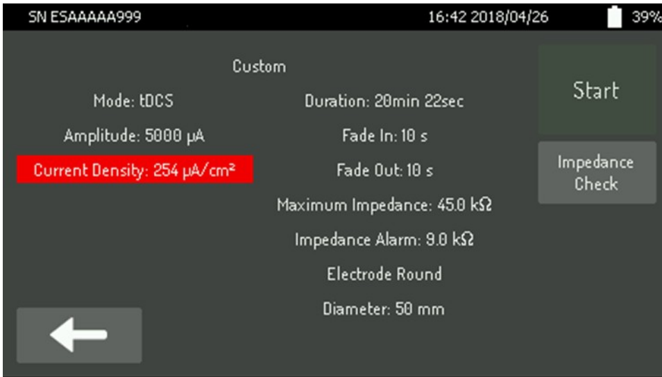
Figure 55. Current density is too high, so stimulation cannot proceed.
